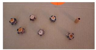
This is a photo of the muscle-bone panels from the front box showing the exit damage of the bullets from the 05152025 testing.
